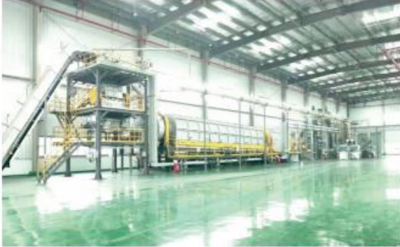
POWER 10KPA Lithium battery breaking and sorting system
