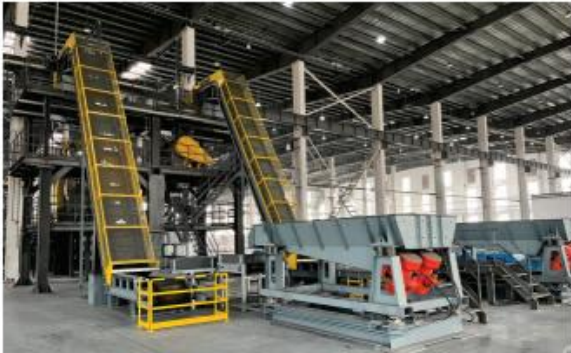
Gotion 250KPA Waste Lithium Battery Breaking and Sorting System
