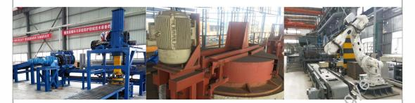
The lead bullion was refined to refined lead or alloy lead. Lead liquid were poured into mold to form lead ingots and stacked automatically. There are standard model and intelligent model.
